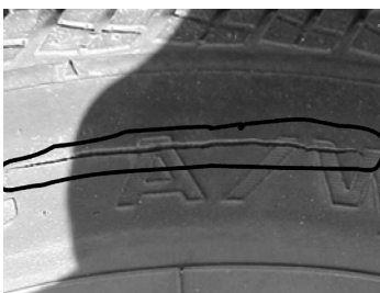
LARGE CRACKS IN SIDEWALL
