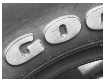
SIDEWALL DISCOLOURATION OR SCUFFING
