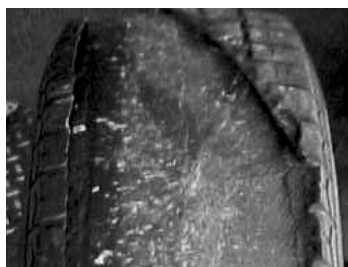
TREAD STRIPPED OFF LINER
