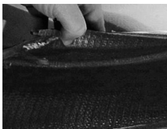
BROKEN OR TORN BEAD
