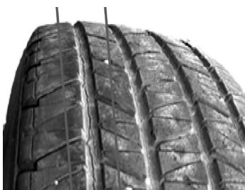
CRACKS IN GROOVE
