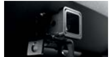
2 INCH RECEIVER Hitch bolts directly into existing holes – no drilling or welding required. 19D520
