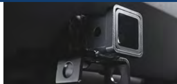
TRAILER HITCH RECEIVER Constructed of tubular crossmembers and finished with a black powdercoat for corrosion resistance. 19D520
