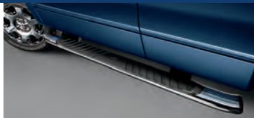
5" STEP BARS – CHROME Corrosion-resistant chrome-plated aluminum tubing is rugged and light weight. 16A450
