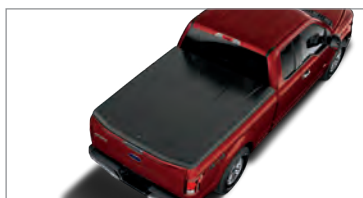
HARD ONE-PIECE BY UNDERCOVER™ FLA Constructed of lightweight ABS polymer plastic compound for strength and durability. 84501A42, 99501A42
